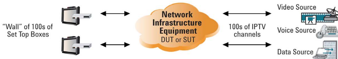
Figure 2: Traditional approach to testing IPTV QoE
