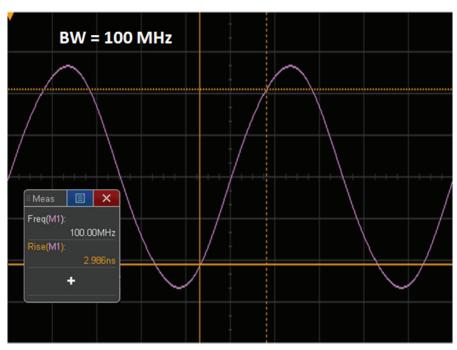
Figure 3: 100-MHz clock captured on a 100-MHz bandwidth scope
