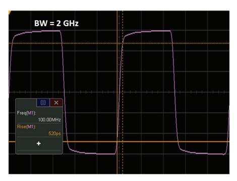
Figure 6: 100-MHz clock captured on a 2-GHz bandwidth scope
