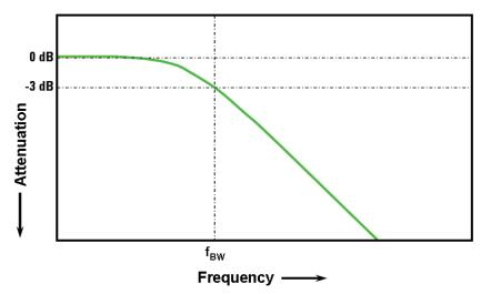
Figure 1: Oscilloscope Gaussian frequency response
