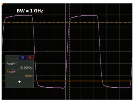
Figure 5: 100-MHz clock captured on a 1-GHz bandwidth scope
