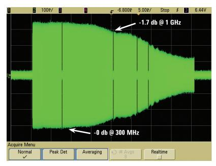
Figure 7: Swept frequency response test on Agilent's MS07104B 1-GHz bandwidth scope
