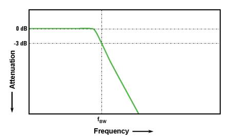
Figure 2: Oscilloscope maximally-flat frequency response
