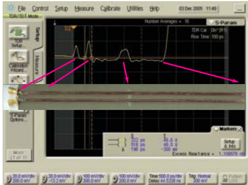
Figure 44. TDR of a single ended transmission line crossing gaps in the return path, showing the inductive discontinuities.
