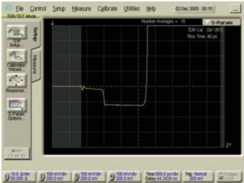
Figure 4. The same transmission line displayed on the impedance scale at 10 Ohms/div, with 50 Ohms in the center.
