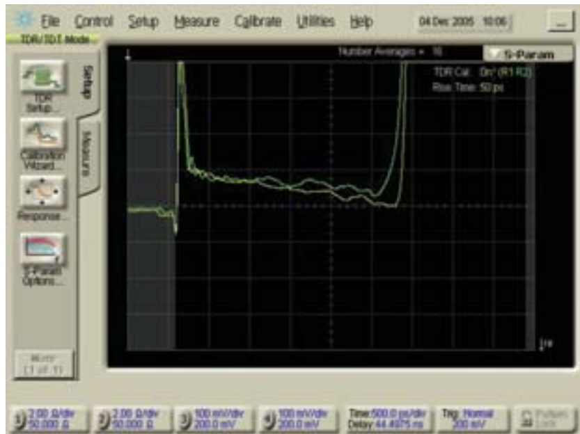
Figure 54. Measured even mode impedance of each line in a differential pair, displayed directly on an impedance scale.
