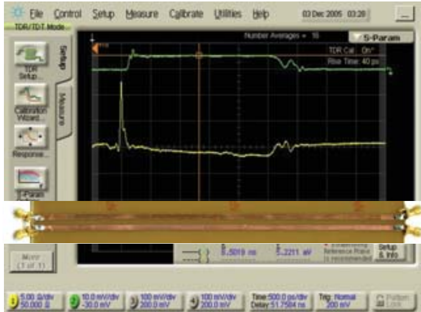
Figure 37. Measurement of the NEXT on a quiet line using the marker.
