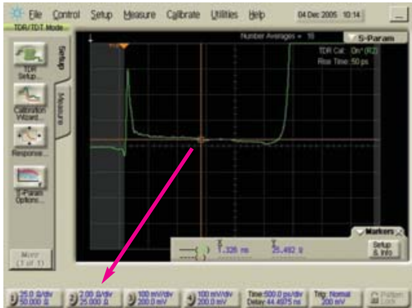
Figure 56. Measured common impedance of a pair of microstrip traces, displayed directly on an impedance scale.
