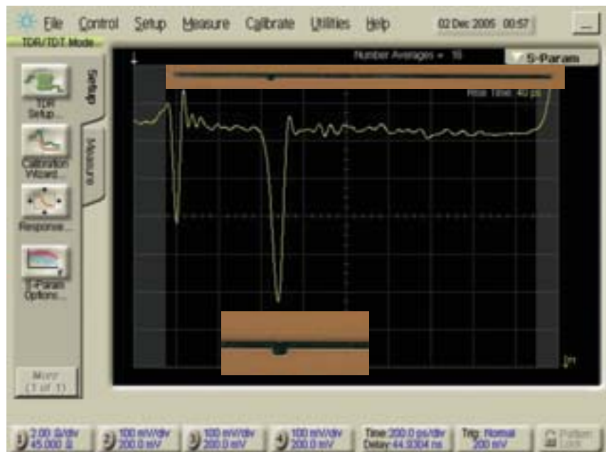
Figure 14. TDR Response from a uniform transmission line having a small test pad.
