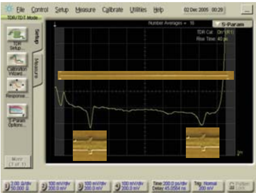
Figure 9. TDR response of a uniform transmission line with two small reference pads, located on four inch centers.
