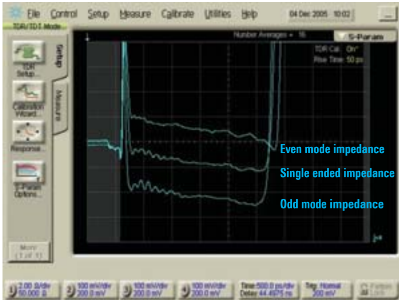
Figure 52. The three impedances of a single line displayed directly on an impedance scale.
