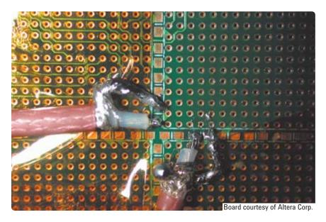
Figure 46. 2-port fixturing of bare circuit board
