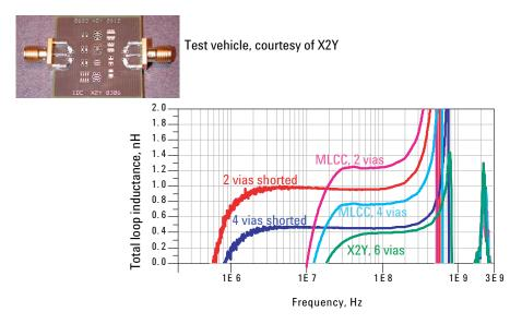
Figure 36. Examples of measured total mounted inductance of capacitors
