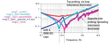
Resonant frequency shifts due to reduction of inductance from no via loop inductance Above board resonance, capacitors don't matter Via loop inductance: Via spreading inductance: Mounting inductance of 4 parallel caps: Mounting inductance of 1 cap:
