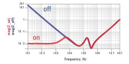
Figure 27. Measured impedance powered on and powered off
