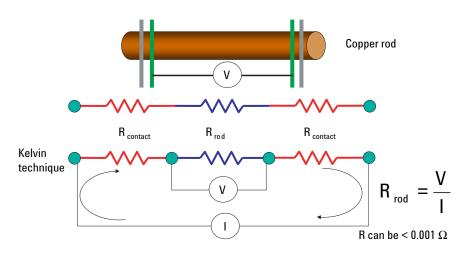
Figure 9. Separate leads for current force and voltage sense eliminate contact resistance effects
