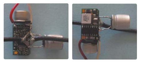
Figure 26. 12 to 1.2 v supply application
