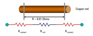
Figure 8. Kelvin technique for a copper rod
