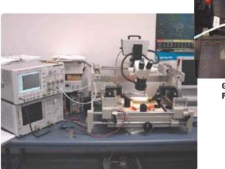
GigaTest Labs PCB probe station
