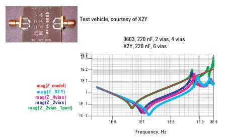
Figure 35. Multiple capacitor samples
