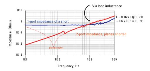
1. Above 100 MHz, impedance is independent of whether the planes are shorted or not 2. Resonances are weak because of the low  $Z_{0}$  of the planes and the  $R/Z_{0}$  attenuation
