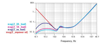
Figure 20. The VRM powered off
