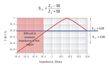
Figure 3. Low impedance measurements can be challenging for 1-port impedance measurements
