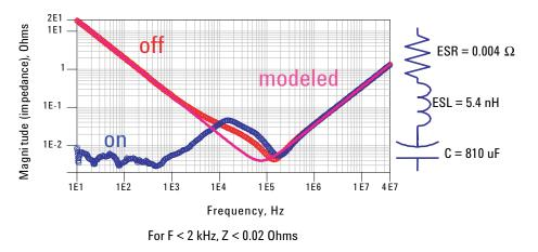
Figure 25. Fitting Simple RLC model to VRM
