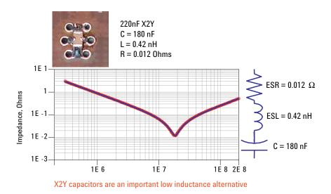
Figure 34. Behavior of real, 200 nF, X2Y capacitor
