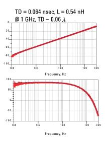
Figure 17. De-embed fixture by modeling
