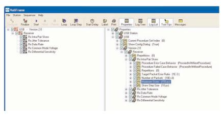
Figure 5: USB receiver intra-pair skew test in expert mode
