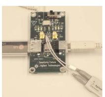
Figure 2: USB fixture with DUT and differential probe
