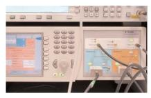
Figure 3: Transition time converters connected to the generator output.
