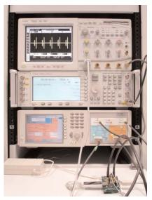
Automated USB 2.0 Receiver Compliance Test and Characterization with the Agilent N5990A Software Platform
