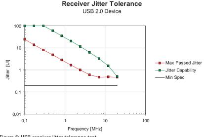
Figure 6: USB receiver jitter tolerance test
