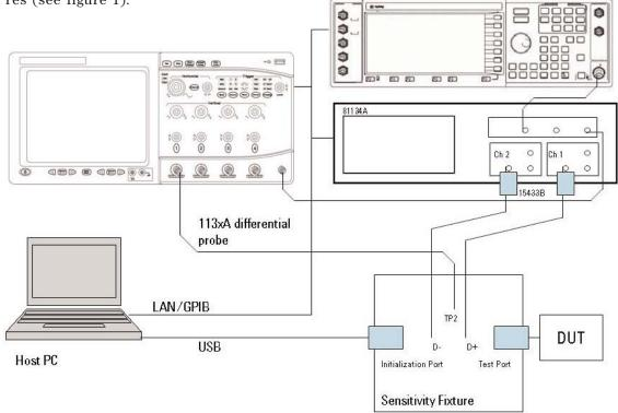
Figure 1 : USB peripheral receiver test setup
