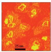
Figure 2. MAC Mode AFM image of the 168-bp circles in 100 µM ZnBr2 / 1 mM MgCl2.
