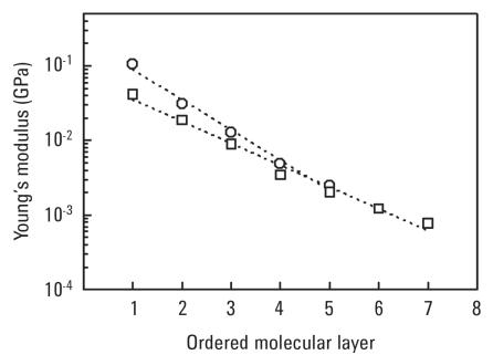
**Figure 4.** The Young's modulus of OMCTS (circles) and mesitylene (squares) at centers of ordered layers. The lines are best-fit lines, indicating exponential decay of the Young's modulus with the number of molecular layers. Data from Figure 2(a) and Figure 3(a).
