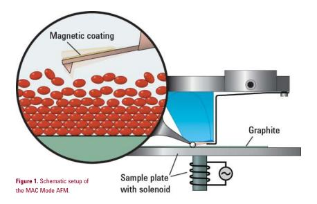
The fluid cell and cantilever holder were thoroughly cleaned before each experiment. OMCTS was always stored in a desiccator filled with  $N_2$  at 4 °C. It was warmed to ambient temperature before being taken out. In each experiment, graphite was cleaved immediately before being covered by fluid. All experiments were carried out at room temperature in air. The characteristics of AFS data presented here did not change over hours of measurements in our experiments.
