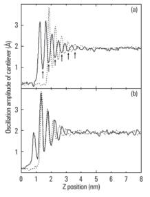
Figure 3. Two typical force spectra at mesitylenegraphite interface in both approaching (solid line) and retracting (dotted line) processes. Up to eight layers of mesitylene were observed. The oscillatory period, 4.4 Å, indicated that the ordered mesitylene rings arranged parallel to the graphite surface. For both (a) and (b): driving frequency = 500 Hz; scan rate = 2.4 nm/sec.
