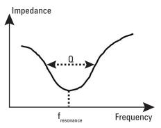
Figure 3. Resonant frequency and Q-factor
