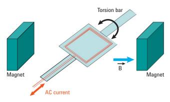
Figure 2. Principle operation of an electromagnetic optical scanner
