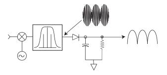
Figure D-1. Peak detector diagram
