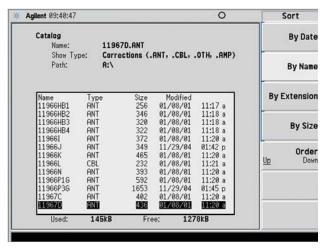
Figure 5. Loading correction factors for a LISN
