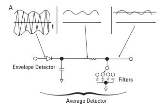
Figure D-3. Average detection response diagram
