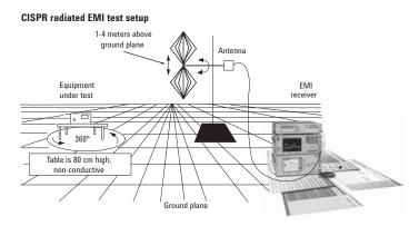
Figure 12. Radiated test setup
