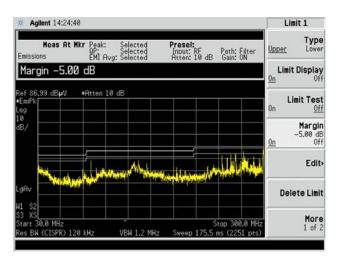
Figure 15. An ambient environment for radiated emissions. Ambients can often be above your limit line. 5.4 Ambient signal measurements
