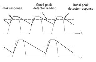
Figure D-2. Quasi-peak detector response diagram
