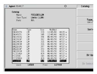
Figure 13. Loading FCC 3-meter class B limit
