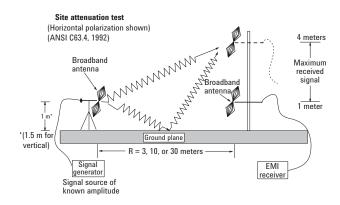
Figure 11. NSA procedure schematic, horizontal polarization
