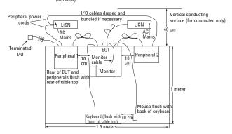
Figure 3. Top view of conducted test setup. The LISN output connects to the receiver.
