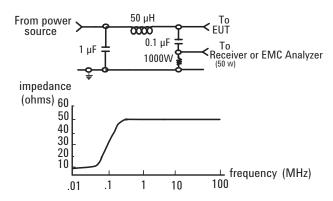
Figure A-1. Typical LISN circuit diagram
