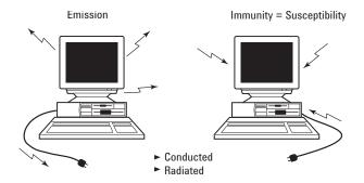
Figure 1. Four types of EMC measurements
