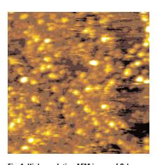
Fig. 1: High-resolution AFM image of S-layer proteins isolated from bacteria and imaged by MAC Mode in liquid.
