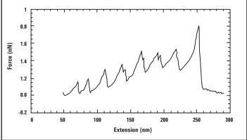
Fig. 5: Left: An AFM image of titin molecules. Right: A saw tooth pattern force-distance curve resulting from the rupture of individual domains of a single titin molecule. The titin molecule was immobilized to a solid surface and then extended between an AFM tip and that surface. Each maxima corresponds to the force required to rupture an individual domain. The distances between the peaks in the curve correspond to the length of each domain.
