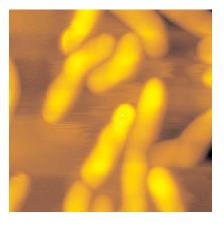
Fig. 2: MAC Mode AFM image of living Rhodopseudomonas palastris bacteria immobilized on a gelatin coated mica surface and imaged in liquid.
