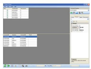
Figure 10 The Power Panel shows a multi-list measurement view of power data in the top table, and ratio and difference computation results between two or more channels in the bottom table.
