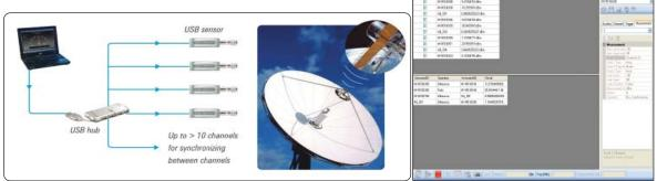
Figure 14 By multiplexing more than ten channels of USB power data with an electronic USB multiplexer, simultaneous data can be obtained from every sensor point and displayed on the versatile Power Analysis Manager.
