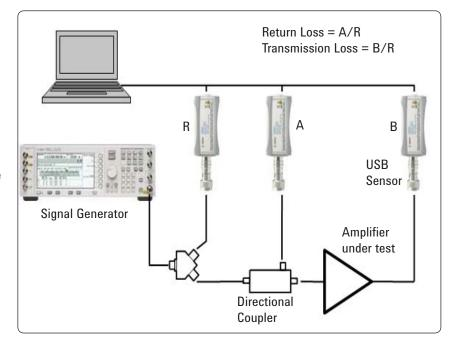
Figure 15 In measurement applications where absolute power data is required, power sensors can measure the absolute output power for assuring compliance and also furnish the power data which permits computing ratios such as return loss and gain, at specified input power conditions.
