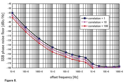
E5052B SSB phase noise floor at 1 GHz (SPD)
