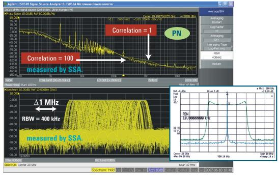
PN example of a drifty signal source (with 2 MHz deviation FM (2 kHz triangle waveform))
