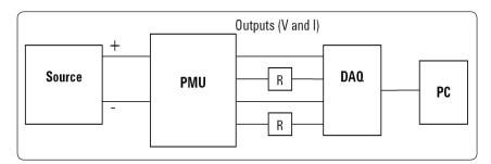
Figure 2. Block diagram shows the test setup of PMU monitoring.
