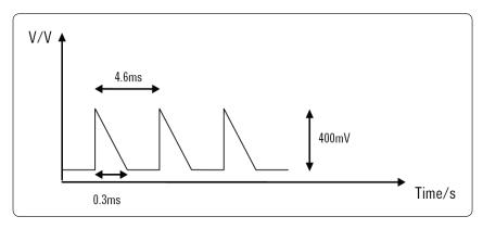
Figure 4. The graph shows an actual glitch detected by the DAQ.
