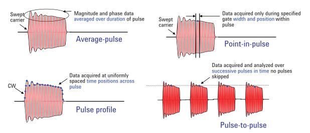
Figure 40. For radar applications, the Agilent PNA has four different pulse-sampling options
