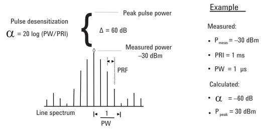
Figure 16. Calculating peak power from the pulsed RF spectrum (line mode) using the pulse desensitization factor
