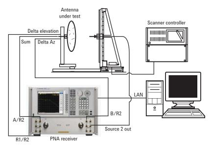
Figure 46. This is an example of a near-field antenna test configuration. Far-field antenna pattern results are extrapolated from the near-field measurements using transformational analysis.
