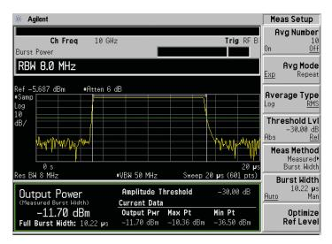
Figure 22. This is an example of burst-power measurement from the PSA spectrum analyzer. Burst power and pulse width are automatically measured in zero-span mode.
