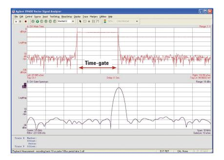
Figure 29. This is a time-gated measurement of simple RF pulse showing CW spectrum of signal when pulse is on
