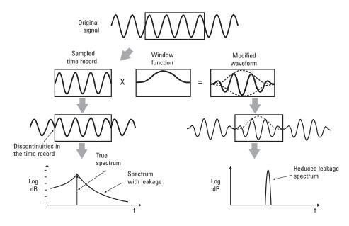
Figure 26. FFT analysis done in a spectrum analyzer or vector signal analyzer assumes a repeating signal. To minimize effects of discontinuities in the signal, a windowing function is used.
