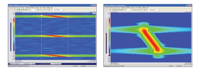
Figure 31. Spectrogram showing chirped radar signal. The left view shows the spectrogram of three consecutive pulses. The right view shows detailed view of a single pulse.
