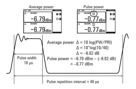
Figure 7. Using an average power meter to derive pulse power.
