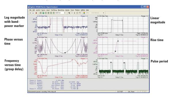
Figure 28. Time-domain measurements on chirp radar using a vector signal analyzer
