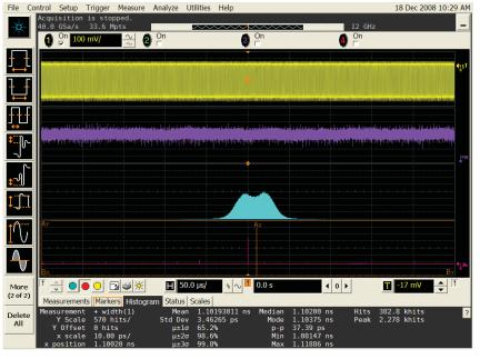
Figure 34. The built-in capabilities of the DSO90000 series make it possible to acquire a chirped radar pulse with a bimodal PRI and then display a histogram of thousands of pulses.
