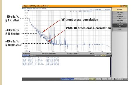
Figure 54. This phase noise measurement uses Agilent's signal source analyzer (SSA). The phase noise measurement is improved using a cross-correlation technique.
