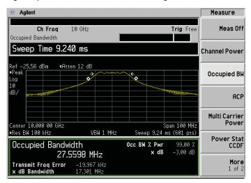
Figure 21. This is an example of an occupied bandwidth measurement on the PSA spectrum analyzer. Bandwidth for which 99.00% of the signal power is contained is automatically measured and reported.
