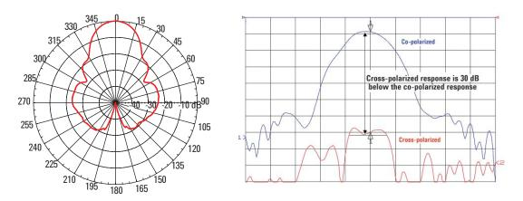
Figure 47. Examples of a far-field antenna pattern and a cross-polarization measurement. The gain can be measured and compared using different polarization orientations of the antenna.
