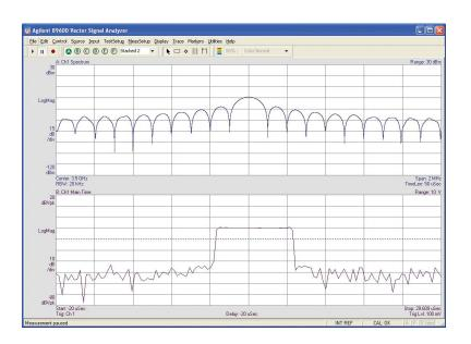
Figure 25. A vector signal analyzer has the ability to provide spectrum analysis of a single pulse.
