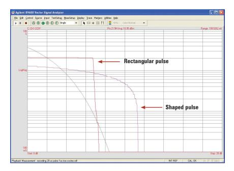
Figure 32. CCDF measurement of a square pulse radar signal compared to a raised-cosine-shaped pulse radar signal. A CCDF plot describes the power statistics of a signal by plotting the percentage of time (y axis) the signal spends at x dB above the average power (x axis).
