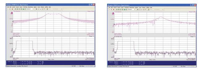
Figure 27. This compares a radar measurement made on a VSA using different windowing functions, uniform (left) and Gaussian (right). The Gaussian window distorts the spectrum because the pulse occurs near the start of the measurement time window. Because pulsed radar signals are selfwindowing, the uniform window function should be used to ensure the best accuracy.
