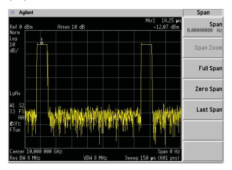
Figure 18. This example of zero-span mode gives a time-domain view of the envelope of the radar pulse. It is a convenient way to measure pulse characteristics when the bandwidth of the radar signal is much less than the RBW of the spectrum analyzer.
