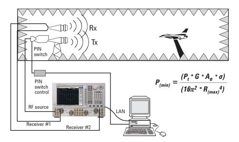
Figure 48. This example radar cross section measurement setup uses a network analyzer and an anechoic chamber.
