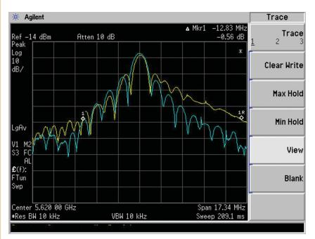
Figure 13. A spectrum analyzer is useful for examining the shape and symmetry of the radar spectrum. This example shows the spectrum trace before and after a timing adjustment in the magnetron.
