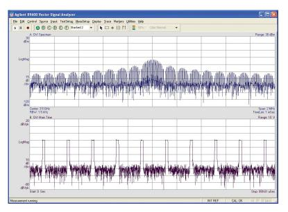
Figure 24. Vector signal analyzer measurement of radar pulse showing spectrum and time domain view
