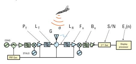
$40Log~(R) = P_{_{T}} + 2G + 20~Log_{_{10}}\lambda + \sigma + E_{_{i}}~(n) + 204dBW/Hz - 10Log(B_{_{n}}) - ~F_{_{n}} - (S/N) - L_{_{T}} - L_{_{R}} - 33dB$
