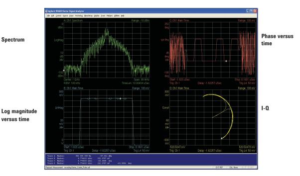
Figure 33. A vector signal analyzer has the ability to examine phase variations over time. This is a useful feature for examining a Barker coded pulse with code embedded in the phase transitions.
