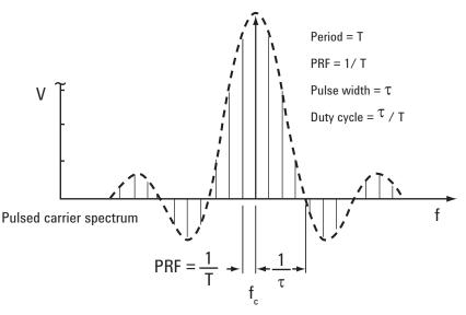
Figure 14. Pulsed spectrum
