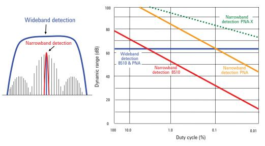
Figure 39. The effects of duty cycle on dynamic range are shown by comparing network analyzer wideband detection and narrowband detection modes
