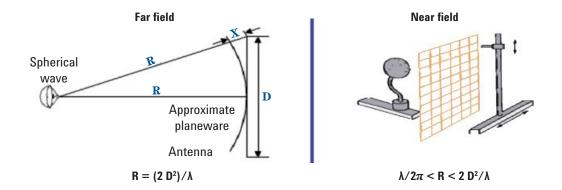
Figure 42. Antenna measurements can be made using either a far-field or near-field approach. Far-field testing is simpler and faster but requires a large area. Near-field testing requires sophisticated calculations and may take longer to perform, but requires less space.
