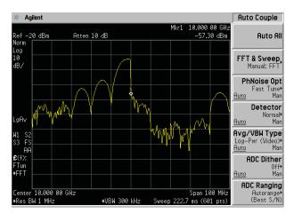
The measurement result may be sporadic when measuring wide band radar signals because the FFT analyzer is required to retune between FFT calculations.
