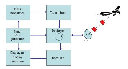
Figure 4. Basic radar block diagram
