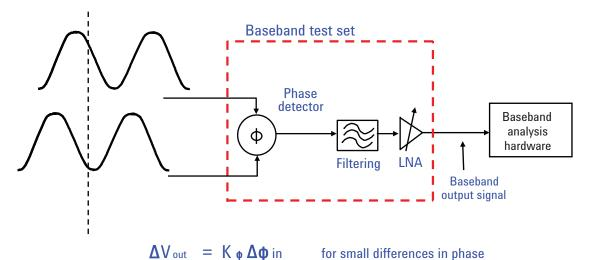
Figure 53. A basic block diagram of phase detector-based phase noise measurement. The measurement compares the test signal to a phase-locked reference signal with a phase detector. Variations in phase due to phase noise result in a voltage output that is then processed to determine the phase noise result.
