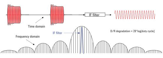
Figure 37. The narrowband detection mode (asynchronous detection mode) of a network analyzer uses a narrow filter to extract only the central spectral component. The narrowband mode has no pulse width limitations.
