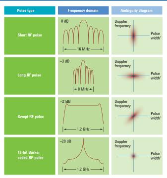
\* The term pulse width on the ambiguity diagram refers to the pulse width at the radar detector output.
