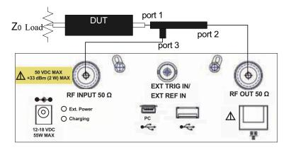
Connect the RF OUT to Port 2 of the directional coupler. Connect the DUT to Port 1. Connect the isolation arm to RF IN. In Figure 3, Port2 and 3 are the isolation ports; port1 and port3 are coupled ports, and while Port1 and 2 are through ports pair.
