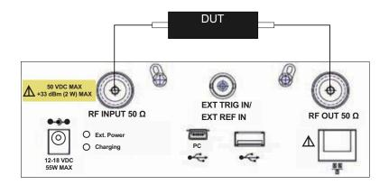
Follow the procedures below to measure the transmission coefficient: Set the frequency, resolution bandwidth, sweep time, input attenuation and tracking output amplitude for the DUT.
