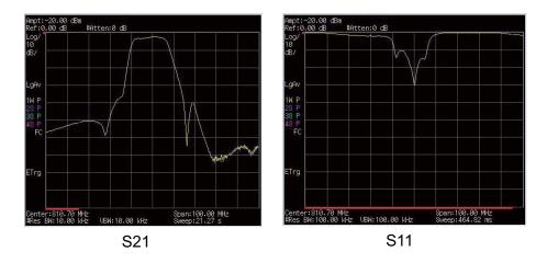
Reflectance measurements often produce errors because of the directivity of directional coupler, a mismatch between source and load impedance, scale fidelity, or normalization of a short or open. A directional coupler with good direction, such as Agilent 86205A with 40 dB high directivity will decrease these errors. Connecting a 10 dB attenuator in series between the DUT and coupler will improve matching.
