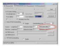
Figure 26. Attenuation level setting
