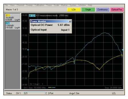
Figure 9. E/O modulation bandwidth measurement
