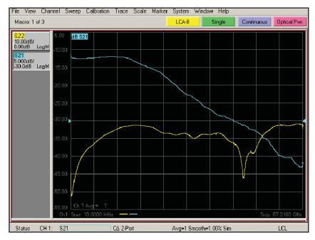
Figure 17. O/E responsivity and electrical return loss measurement
