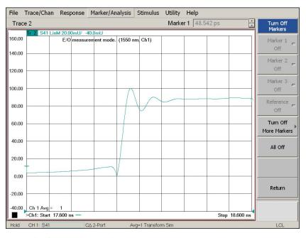
Figure 13. E/O step response of laser
