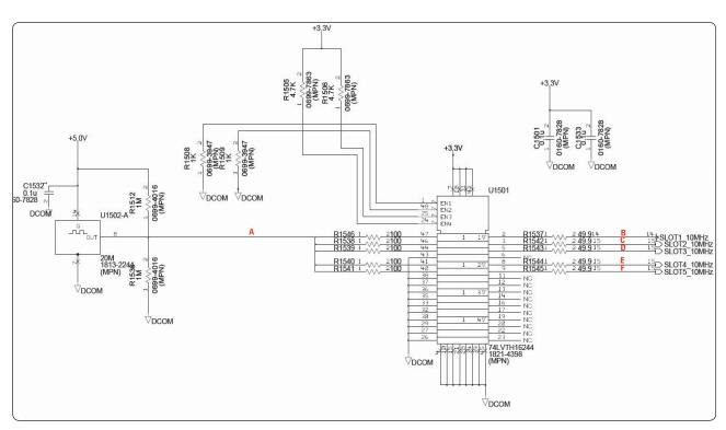
Figure 4. Reference clock schematic for carrier board
