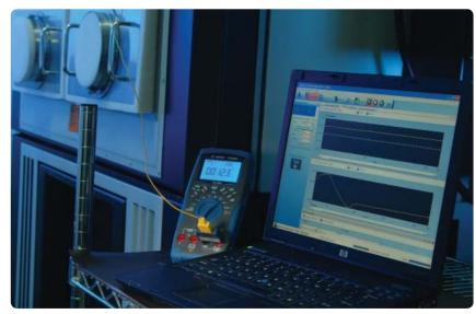
Figure 1. Performing data logging with the U1250A Series handheld DMM and the GUI datalogger software.
