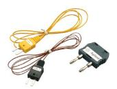
Thermocouple adapter is a cost effective solution to your temperature measuring needs. The Agilent U1180A thermocouple adapter and lead set includes a non-compensation transfer adapter, J-type and K-type thermocouple beads. The transfer adapter is used to convert the thermocouple's miniature connector to banana plugs (for adapting to the DMM's terminal). Both thermocouple J-type and K-type have effective temperature range of  $-20~^{\circ}\text{C}$  to 200  $^{\circ}\text{C}$ .
