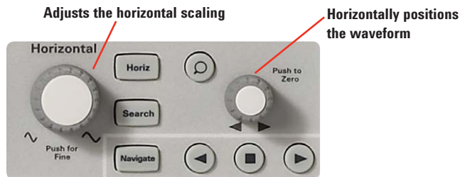
Figure 17. Front panel horizontal control section on an Agilent InfiniiVision 2000 X-Series oscilloscope
