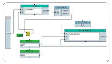
Figure 8. Exponential averaging and linear calibration of TPS value
