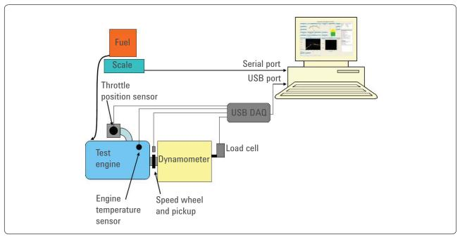
Figure 1. Schematic overview of test system
