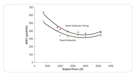
Figure 12. Brake-specific fuel consumption vs. engine power for stock and tuned carburetor
