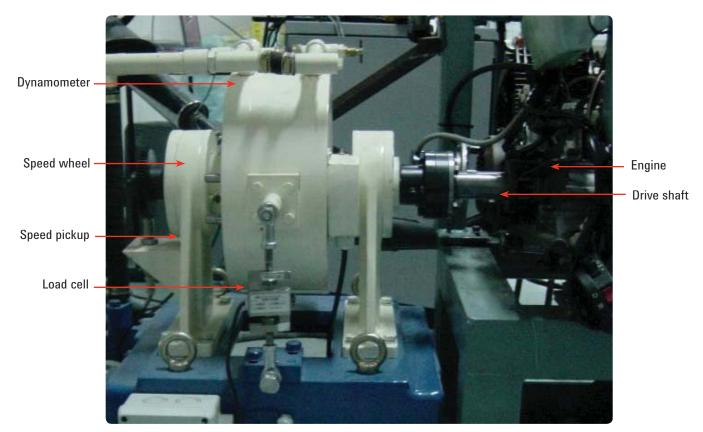
Figure 7. Side view of dynamometer and engine
