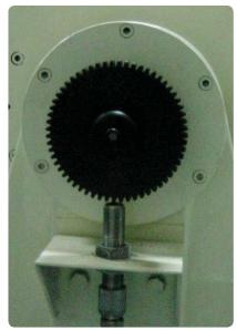
**Figure 4.** Speed wheel (top) and pickup (below)
