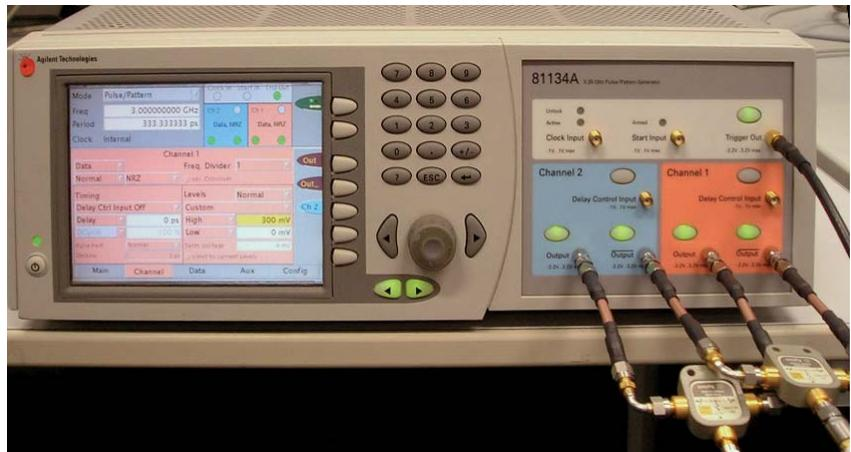
Figure 1: the Agilent 81134A Pulse Pattern Generator connected to two times 11636B power dividers.
