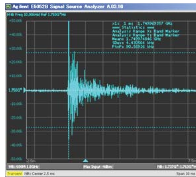
Figure 11. Modulated RF signal behavior by external mechanical stresses
