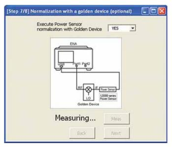
Figure 14. Normalization using golden device
