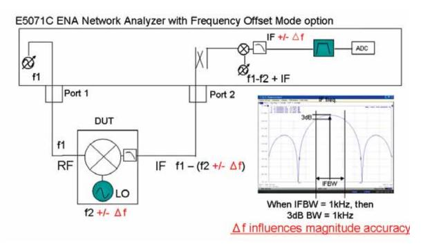
Figure 1. IFBW vs. LO frequency drift with FOM
