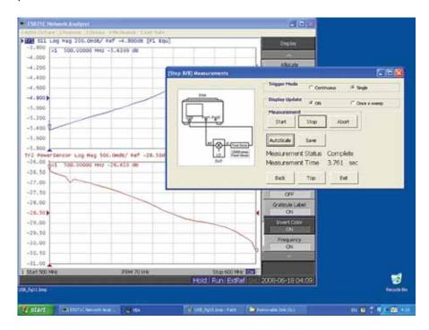
Figure 16. S11 (Trace 1 in blue) and power meter (Trace 2 in red) frequency sweep
