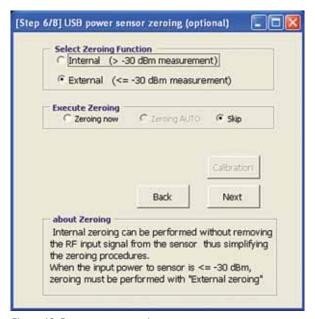
Figure 13. Power sensor zeroing
