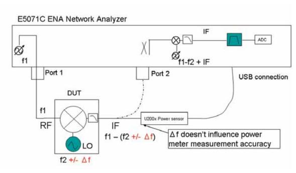
Figure 2. Power sensor (broadband detect) vs. LO frequency drift
