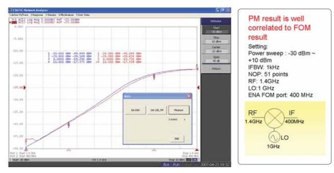
Figure 3. Measurement results with Locked LO (RF Power vs. IF Power)
