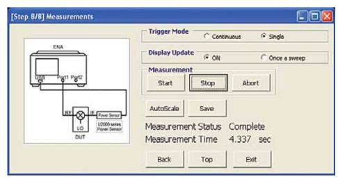
Figure 15. Measurement window
