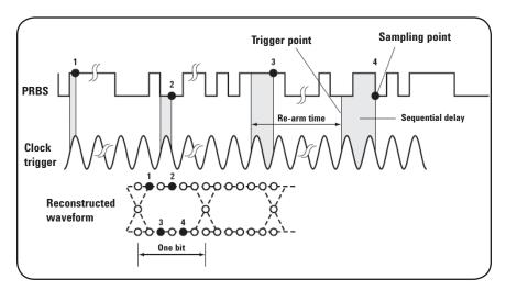
Figure 4 - Sampling Process for an Eye Diagram Waveform
