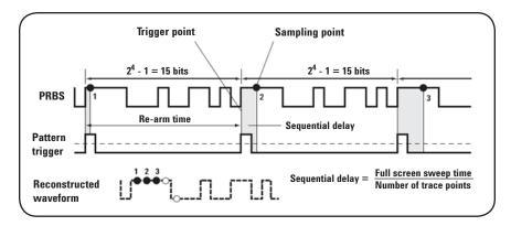
Figure 3 - Sampling Process for a Bit Steam Pattern Waveform
