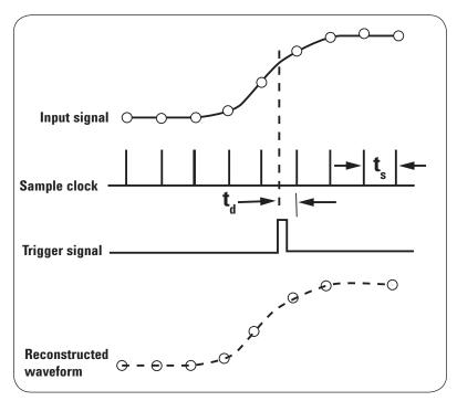
Figure 1 – Waveform acquisition using a real-time oscilloscope
