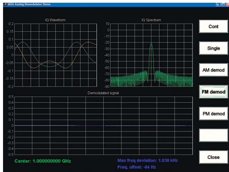
Figure 9. Example of program using MATLAB's GUI capabilities
