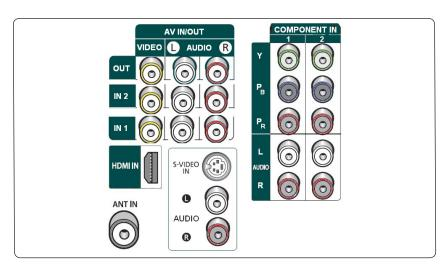
Figure 1. Typical types of TV connectors
