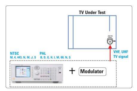
Figure 6. Antenna RF input test setup
