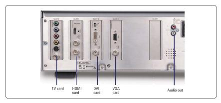
Figure 3. U8101A display tester with configurable plug-in cards
