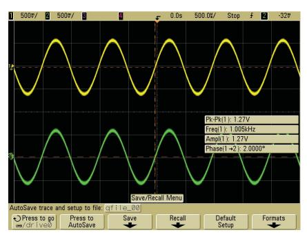
Figure 4. Oscilloscope with built in Vp-p and phase relationship measurement
