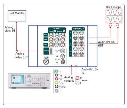
Figure 2. The diagram for AV test setup
