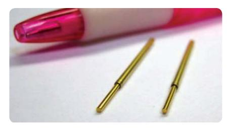
Figure 4 : Headless test probes were used on bead probe locations.
