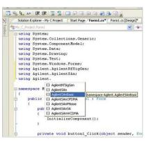
Figure 2. Depending on the context, the Intellisense popup window will show available drivers or installed drivers.
