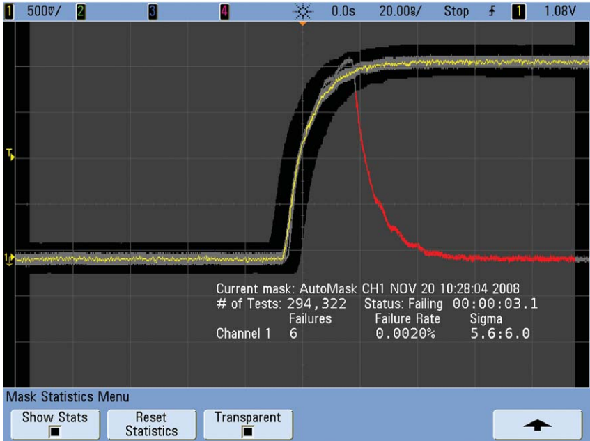
Figure 5. Mask tests make it easy to observe when a signal fails the QA process
