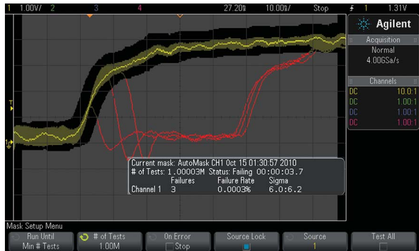
Figure 6: Mask testing to 6.2 \sigma resolution takes only seconds using an InfiniiVision scope with a mask test rate of 270,000 waveforms tests per second
