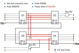
Figure 3. Interconnect Test checks connections for most shorts and some opens within the chain.
