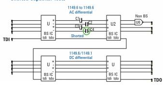
Figure 8. Agilent Medalist i3070 interconnect test and shorted capacitor test on 1149.6 DC/AC differential signals.
