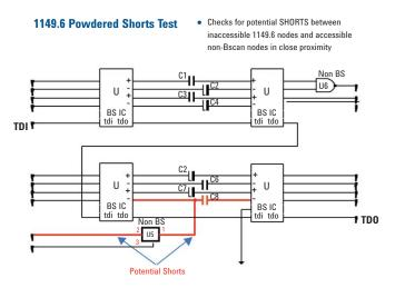
Figure 10. Agilent Medalist i3070 Powered short test on 1149.6 DC/AC differential signals.
