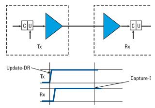
Figure 2. Typical 1149.1 output and input boundary scan cell connection.
