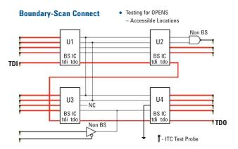
Figure 6. Connect Test checks the connections of each device in a chain.
