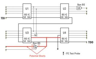
Figure 4. Agilent's Powered Shorts test checks for shorts between boundary-scan nodes without test probe and any nearby non Boundary Scan node with test probes.
