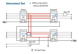
Figure 5. Bus Wire Test verifies connections on bussed nodes.
