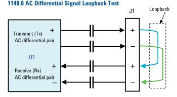
Figure 12. 1149.6 AC Differential Loopback testing
