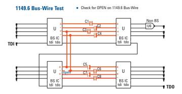
*Figure 9. Agilent Medalist i3070 Bus wire test on 1149.6 DC/AC differential signals.*
