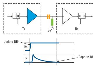
AC Coupled signals that decay before they can be captures
