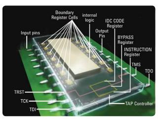
Figure 1. A boundary scan device
