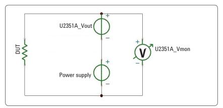
Figure 2. Schematic circuit for U2351A connectivity with DUT
