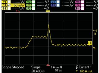
To achieve the ramp rate requirements for V<sub>CCINT</sub> and V<sub>CCO</sub> (see Figure 1), the slew rates for channels 1 and 2 were adjusted. **Figure 4** shows the N6705A display for changing a channel's slew rate, which is expressed in volts per second (V/s). Below the slew rate settings screen is the rising slew rate of channel 1 and 2 on the N6705A outputs. The rise time is captured using the markers for the display.
