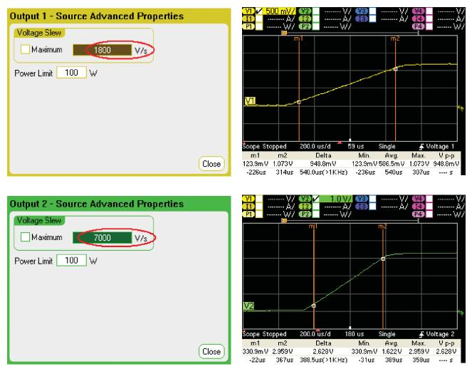
Figure 4. Core voltage and I/O voltage slew rate settings
