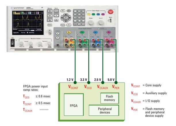
Figure 1. FPGA circuit test setup
