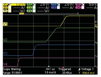
Figure 5. Power module voltages at turn-on
