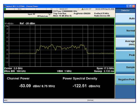
Figure 7. RF spectrum for Pedestrian B fading.
