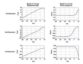
FIGURE 2: The X-parameters are shown here overlaid on actual circuit-level PA results. As is evident, the X-parameters accurately correlate with the actual circuit.
