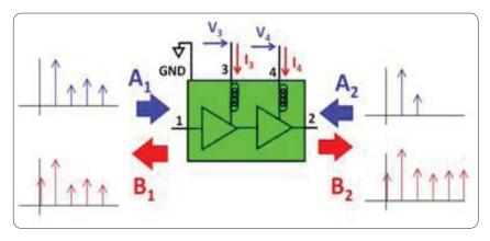
FIGURE 1: The X-parameter model for the multi-stage amplifier in this example is formulated in the frequency domain and maps incident waves (A) to scattered waves (B). Because the complete knowledge of magnitude and phase of incident and scattered waves at all harmonics is exactly equivalent to complete knowledge of the time-domain waveform, the full nonlinear input-output characteristics of the device are captured.
