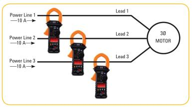
Figure 2. Motor under normal condition
