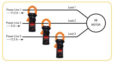
Figure 3. Motor under single-phasing
