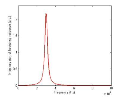
Figure 6. The imaginary part of the frequency response comes entirely from the odd part of the time response (Figure 2, in this case). Note that for aesthetic reasons, the curve was flipped up-down. The imaginary part is actually negative. Physically, the peak corresponds to severe damping at the resonant frequency (30 MHz).
