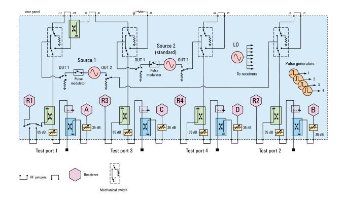
FIGURE 1: Block diagram of the PNA-X N5242A Option 423 RF test set.
