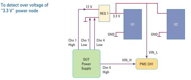
Figure 4. PMC connection to detect over voltage
