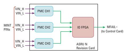
Figure 1. Power monitoring circuit (PMC) block diagram
