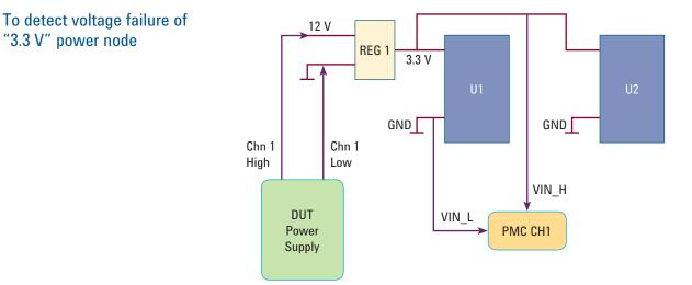
Figure 3. PMC connection to detect voltage failure
