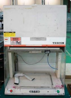
a table that is provided by the user. All other mechanical aspects of the press down unit are similar to the i1000D system. The system runs on an old MS DOS PC controller which makes integration of today's 3rd party software almost impossible.
