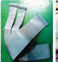
Figure 5. 64-pins to 32-pins split flat cable
