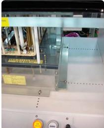
Figure 7. Spacer bar added between bar and fixture.
