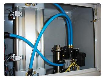
Figure 11. Adjust the lower sensor to lit position
