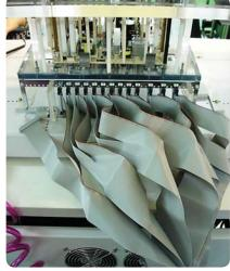
Figure 6. Tescon fixture connected to i1000D
