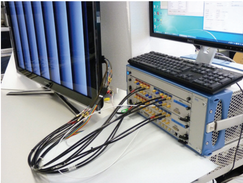
Figure 7. Example sink test setup using M8190A AWG
