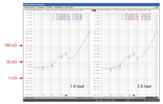
Figure 31. DC-DC converter output impedance measurement
