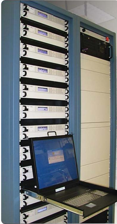
Figure 12. The rack on the left uses 12 Agilent E4360A SAS units to deliver 24 channels of simulation
