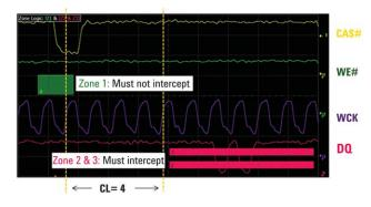
Figure 3: Separate Read command with InfiniiScan+ zone qualify trigger tool
