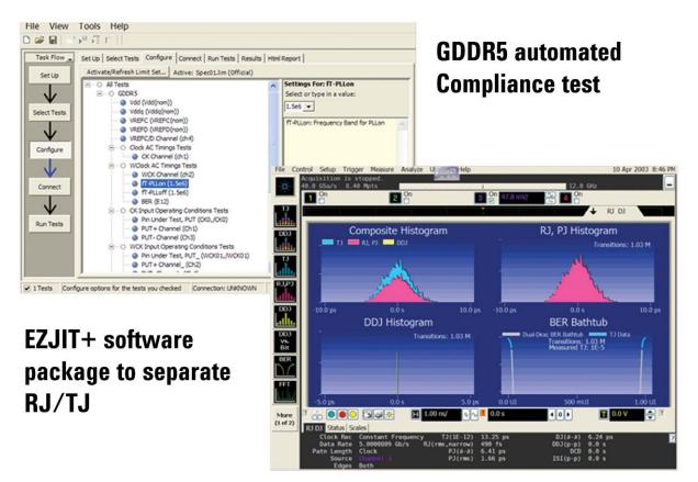
Figure 1: The 90000X series true analog bandwidth oscilloscope is a tool of choice to separate TJ/RJ measurement with an automated compliance test application with EZJIT+ jitter tool.
