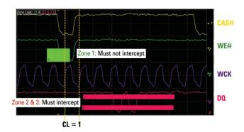
Figure 4: Separate Write command with InfiniiScan+ zone qualify trigger tool
