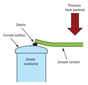
Figure 7. A piece of small debris is stuck on the surface of center conductor
