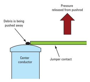
Figure 8. Debris is being pushed away by wiping process of the jumper contact
