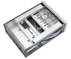
Figure 21. Sample in-house switch matrix design
