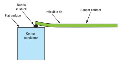
Figure 5. Particle buildup remains trapped between the jumper contact and center conductor
