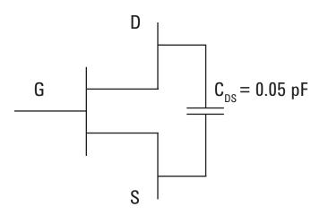
Figure 1. GaAs MESFET Schematics and Equation
