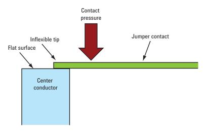
Figure 4. Conventional electromechanical switch mating configuration
