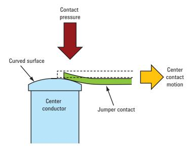
Figure 6. Electromechanical switch mating configuration illustrating microscopic wiping
