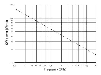
Figure 11. Power rating for cold switching at 75 o C
