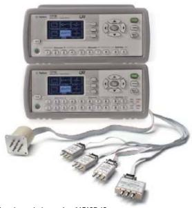
Figure 13. Driving the switches using 11713B/C
