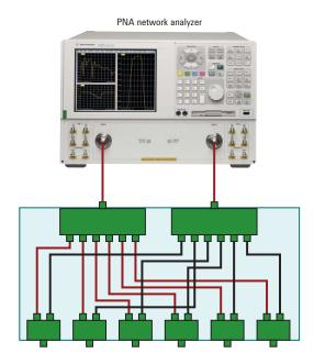
Figure 9. PNA network analyzer with a multiport test set
