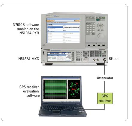
FIGURE 1: Shown here is a typical GPS receiver test setup with the N7609B. The baseband GPS signal is created by the N7609B running on the N5106A PXB, upconverted to RF by the MXG and sent to the GPS receiver. The GPS receiver output is then sent to evaluation software on a PC.
