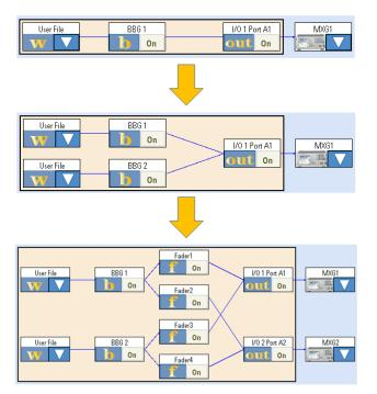
FIGURE 2: The PXB can be easily reconfigured in software to provide different test capabilities. This diagram shows three different possible configurations: single-channel signal generation for creating one format such as GPS, 2-channel generate and sum for interference testing using a single RF signal generator, and 2x2 MIMO with 4 channels of fading for testing MIMO formats such as LTE and WiMAX.
