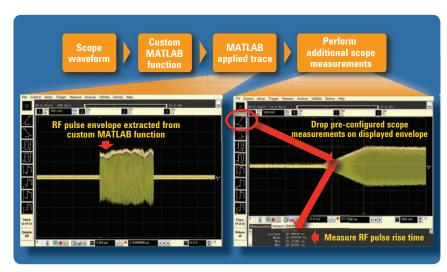
FIGURE 2: Pulsed RF envelope and rise time measurements performed on the envelope.
