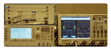
FIGURE 1: Shown here is the typical hardware test setup used to create and analyze wideband Radar and Satcom signals. An M8190A wide bandwidth AWG is shown on the upper-left, a PSG with wideband I/Q inputs is shown on the lower-left, and a wide bandwidth 90000 X-Series oscilloscope with VSA software is shown on the right.
