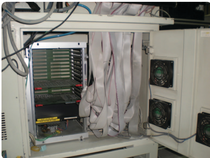
Figure 2. Functional module rack installed in the card cage
