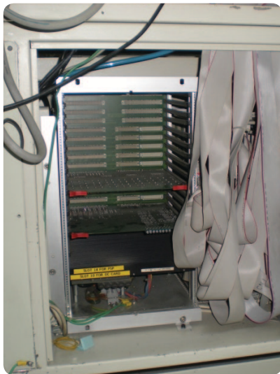
Figure 3. Functional rack installation in card cage reduces usable card slots
