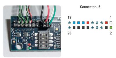
Figure 1. Connections on CET card (J6 connector)
