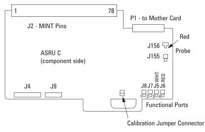
Figure 2. Connector locations on ASRU Card
