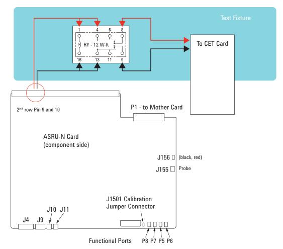
Figure 6. Fixture power supply isolation from system ground
