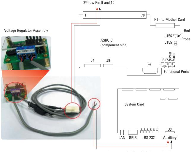
Figure 4. Wiring of Aux #5 to voltage regulator assembly
