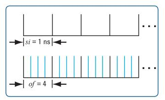
Figure 2. Oversampling by a factor of 4 within a 1-ns sampling interval yields an effective sampling rate of 4 GSa/s
