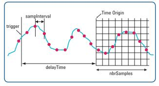
Figure 3. The acquired waveform can be positioned in time using sampling interval and delay time
