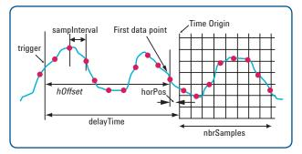
Figure 4. Sub-bins are created by random variation in horizontal position (horPos) relative to the waveform.
