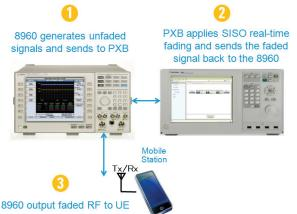
FIGURE 2: With the single-channel (SISO) test configuration, single-channel fading is applied to the 8960 for user equipment testing.
