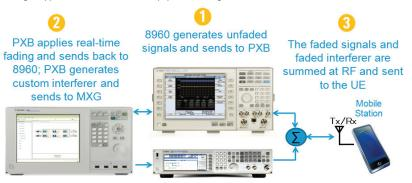
FIGURE 3: With the single channel with custom interferer test configuration, the PXB applies real-time fading to the 8960 and generates custom interferers.
