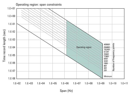
Figure 4. The allowable range of spans, which may differ by model, further bound the operating region of the oscilloscope.
