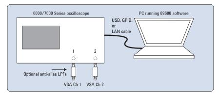
Figure 1a. Equipment connections for 2-channel oscilloscopes
