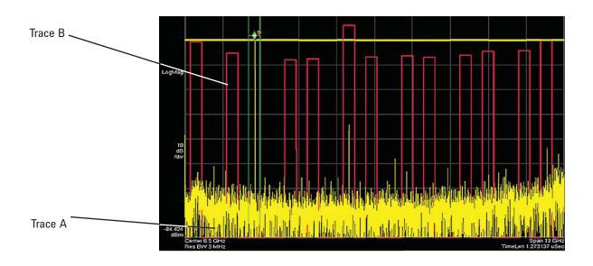
Figure 7. Alias Exposure Zone Checker results. The desired signal is at 2.38 GHz. The unwanted signal in the fifth alias zone at 5.62 GHz is over 5 dB above the threshold line, shown in yellow here.
