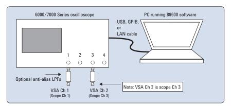
Figure 1b. Equipment connections for 4-channel oscilloscopes when using 2 VSA channels<sup>1</sup>
