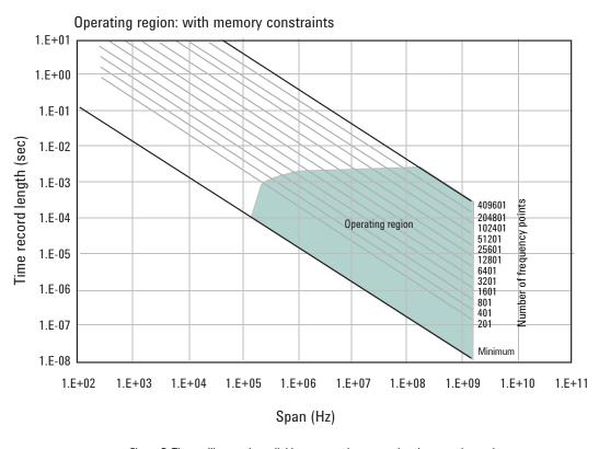
Figure 5. The oscilloscope's available memory also constrains the operating region.
