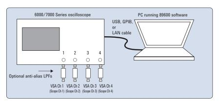
Figure 1c. Equipment connections for 4-channel oscilloscope used to provide 3- or 4-channel VSA measurements using the 89600 VSA software.<sup>1</sup>
